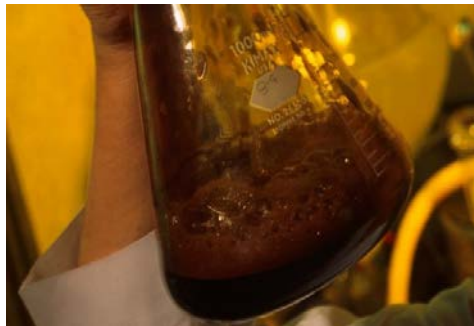
Figure 4 "Brown liquor" Sulfite waste liquor from paper industry: Fermentation leads to Torula yeast
