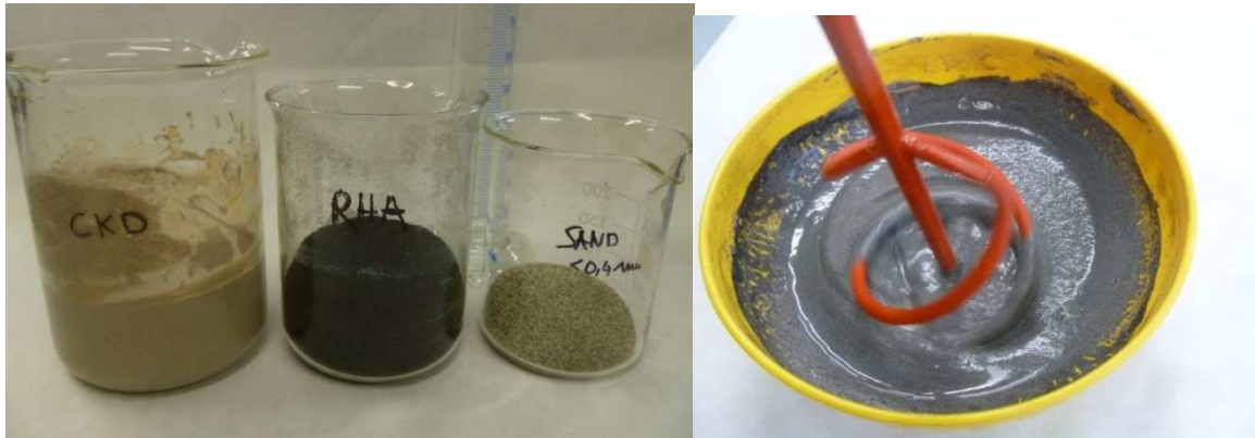
Blending of the Ecocement components: CKD; RHA; Sand; Urea Solution and Biomass
