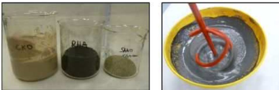
Blending of the Ecocement components: CKD; RHA; Sand; Urea Solution and Biomass
